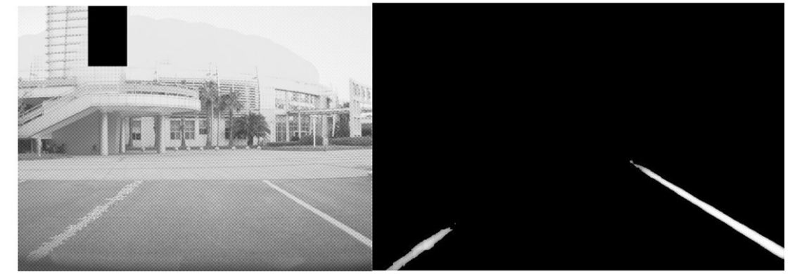
Fig 30. Left picture shows we add some patch around the left lane line in digital level, and right picture shows the result
