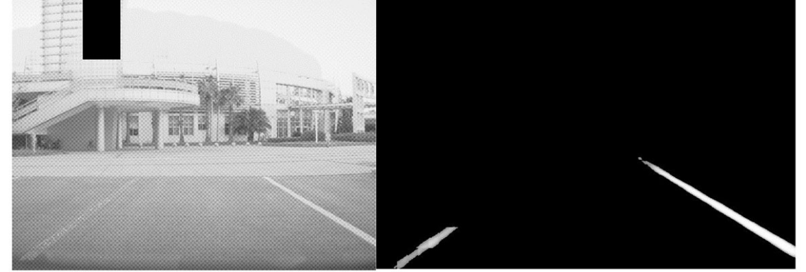
Fig 29. Left picture shows we add some noise on the left lane line in digital level, and right picture shows the result of APE's lane recognition function. (We redact top left of our image for privacy reasons, but it won't affect the final result.)
